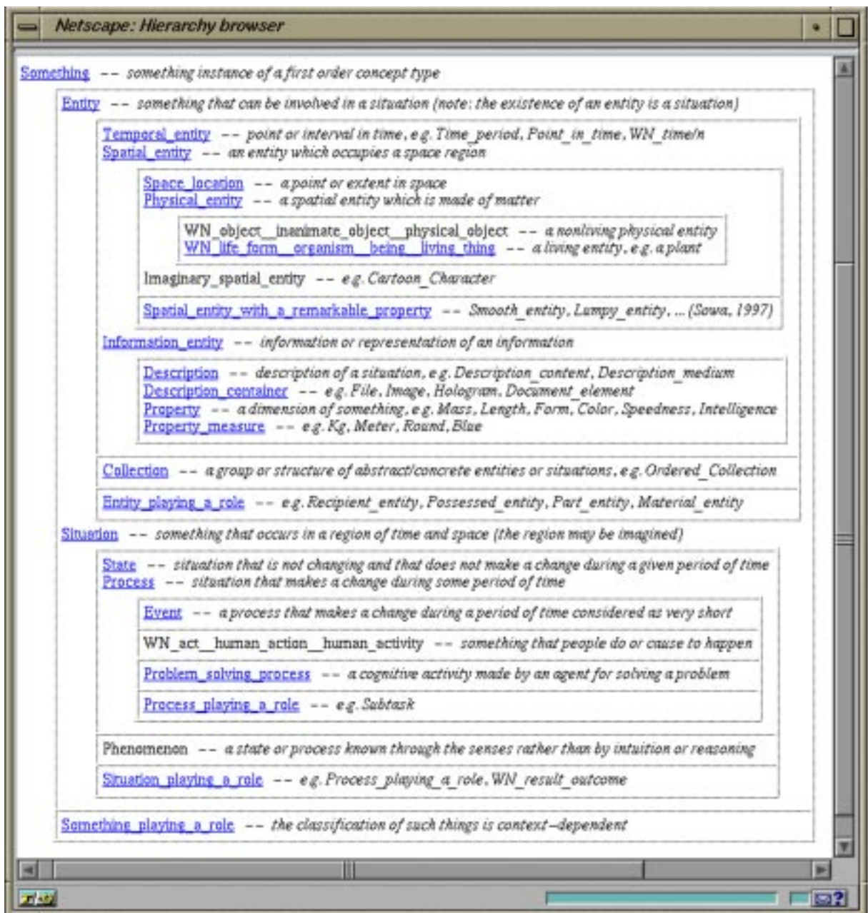
Fig. 10. Uppermost concept types of the WebKB top-level ontology (types at the same level in a same box are exclusive; types beginning by WN come from the WordNet ontology).
